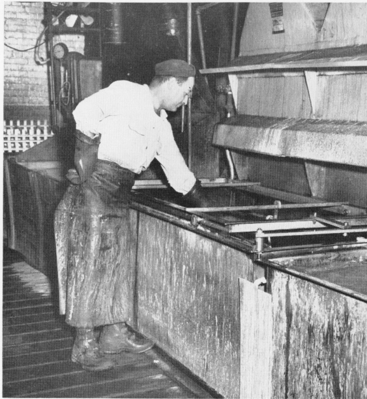
Mike Walker of the Aluminum Finishing Department is about to remove a rack of work from a tank containing hot concentrated acid solution which is used for brighten-
